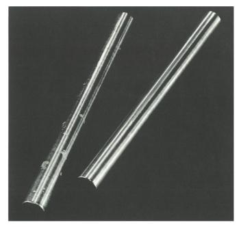
These two bars are immersed in quiet seawater for nine months. The bright shiny bar above is AK Steel's ARMCO NITRONIC 50 Stainless Steel and at left is Type 316 stainless steel showing considerable pitting and crevice corrosion.
